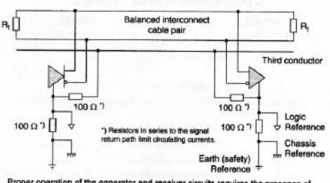
Proper operation of the generator and receiver circuits requires the presence of a signal return path between the circuit grounds of the equipment at each end of the interconnection
