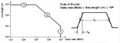
Maximum Data Rate in a Balanced Interface
