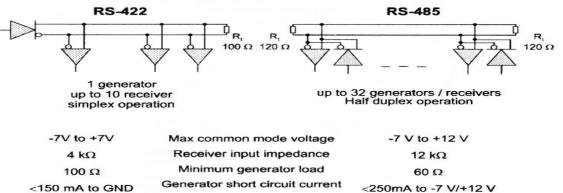
This picture compares the standards RS 485 and RS 422, summarizes individual values and shows connections of termination resistors.
